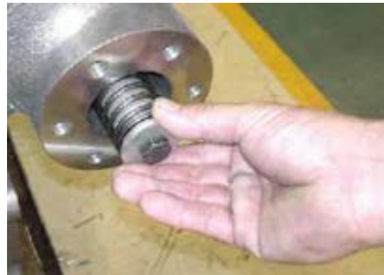
Unloader (device spring and push rod)
