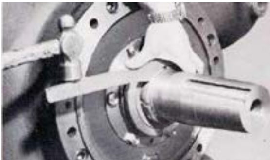
Special tool for loosening the seal collar lock nut
