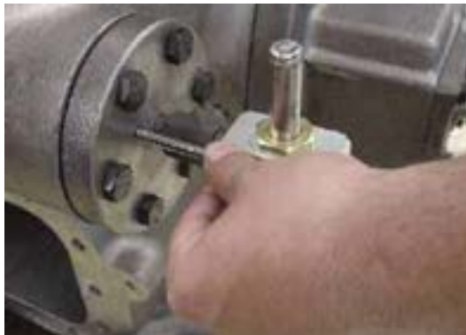
Adjustment of push rod position
