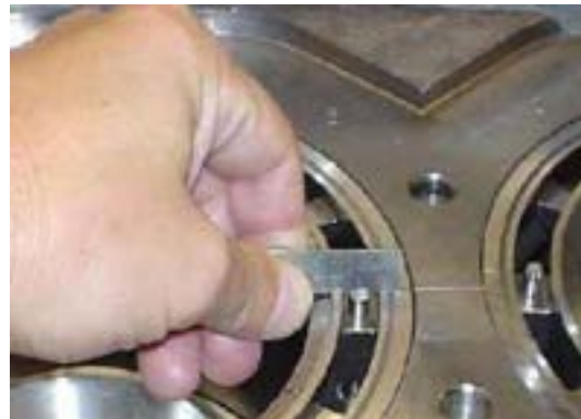
Adjustment of lift pin height
