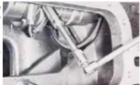
Removal of valve plate
