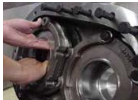
Removal of valve plate
