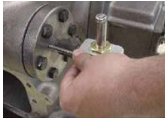
Position adjustment of the unloader push rod
