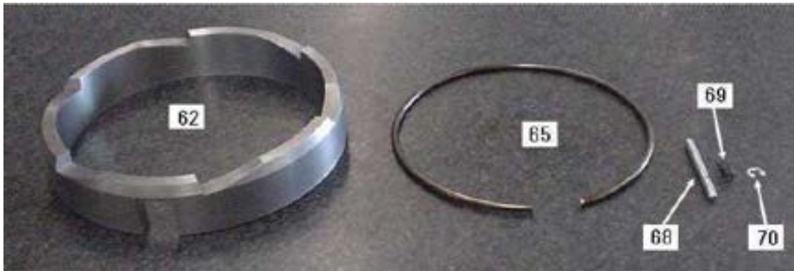
Unloader components (to be attached to the cylinder sleeve)
